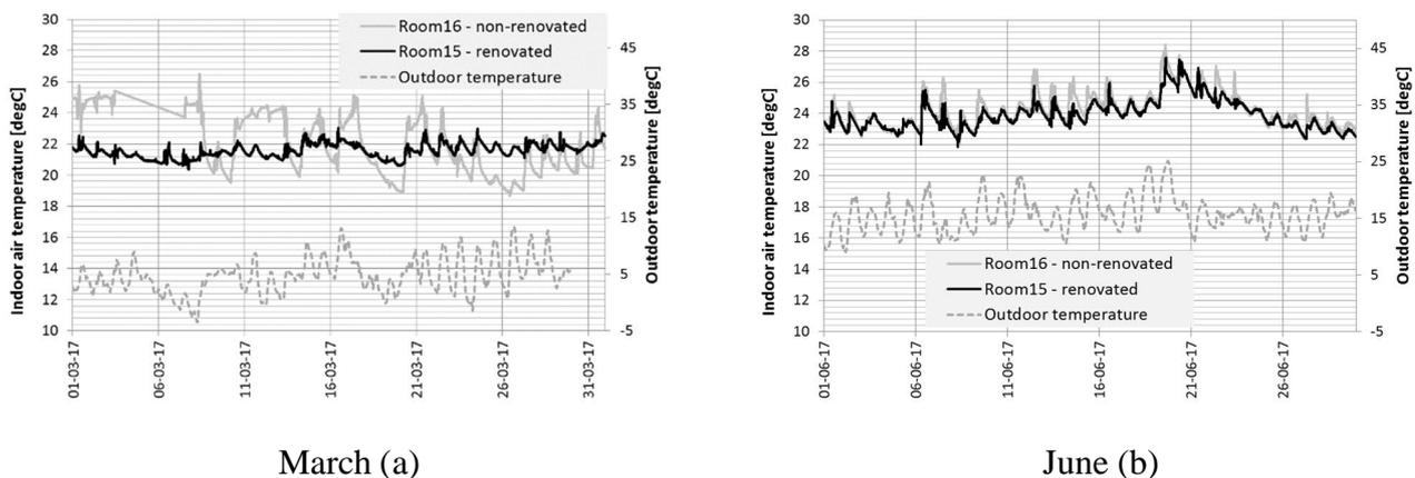
Figure 4. Indoor air temperature in March (a) and June (b) in the classrooms (solid lines, left y-axis) along with the outdoor temperatures (dashed line, right y-axis).
